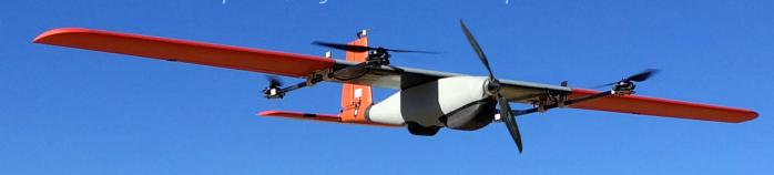
Lynx VTOL is a vertical takeoff and landing drone for precision agriculture and surveying. Lynx VTOL blends the ease-of-use of a multicopter with the endurance of an airplane. Takeoff and land as a copter; fly the mission as an airplane.
